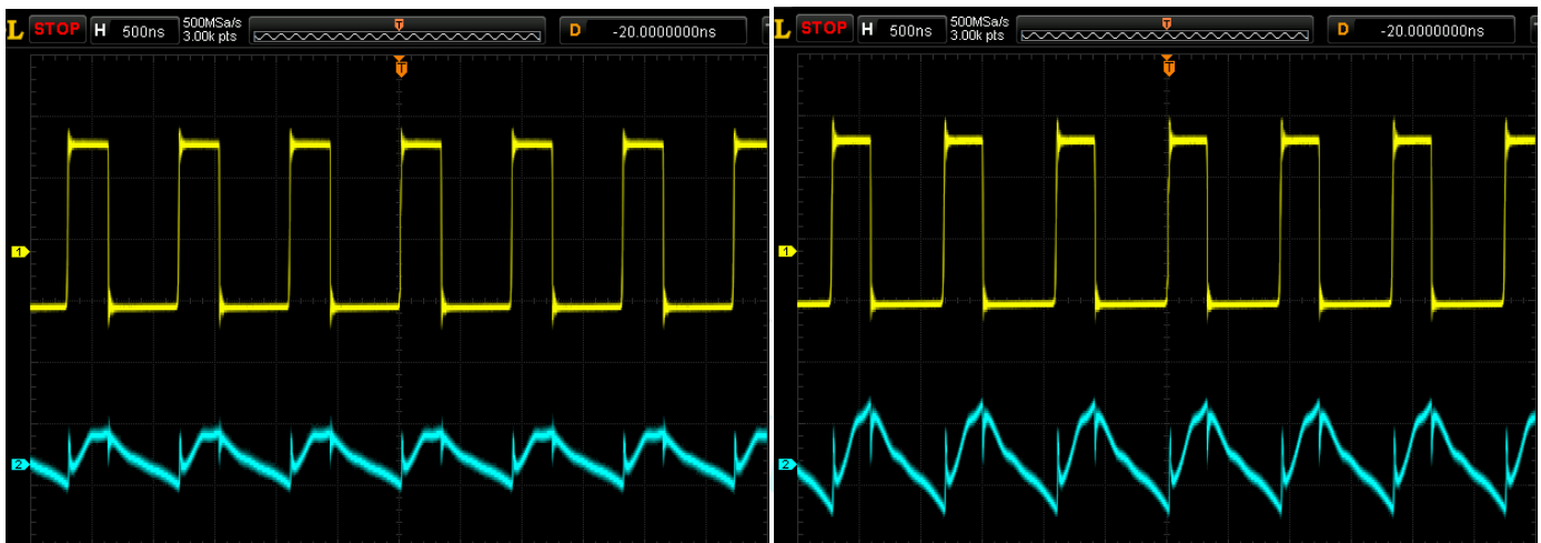
V_{IN}=5V, V_{OUT}=12V, I_{OUT}=300mA, CH_1=V_{SW}, CH_2=\Delta V_{OUT}
