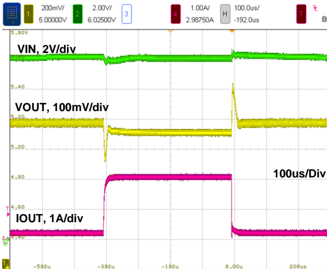
Figure 27. Load Transient, 0.2A-2A-0.2A
