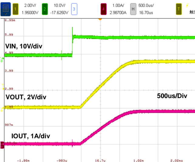
Figure 15. Startup by VIN, 3Ω load
