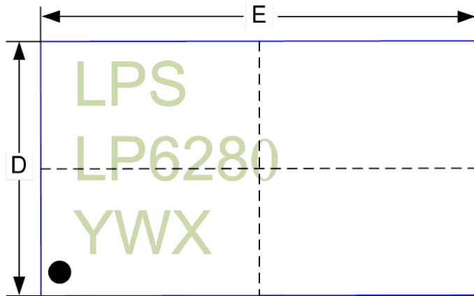
WLCSP-15-ball Package (1.17×1.94) pitch 0.4 (Unit: mm)
