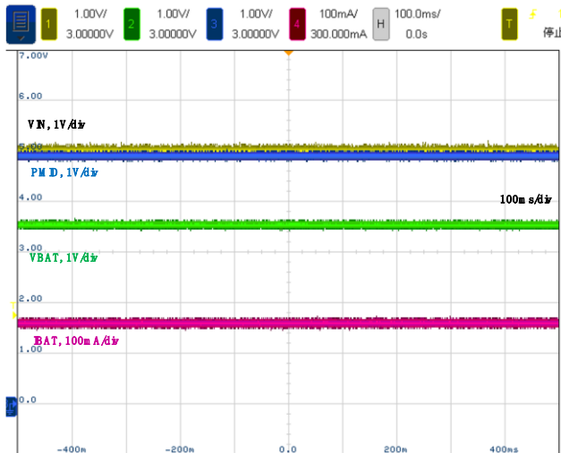
Figure 21. Charge with low ICC, ICC=150mA
