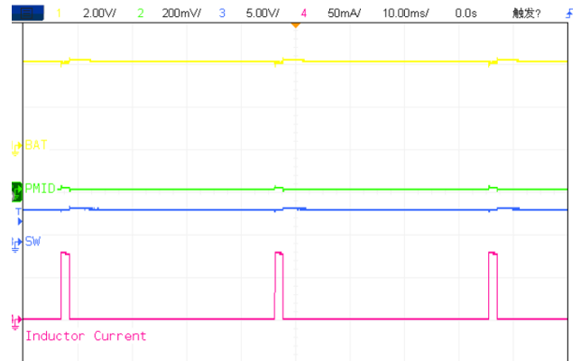
Figure 16. Switching waveform, VIN=4.0V, short circuit protection
