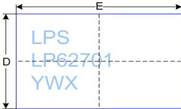
WLCSP-15-ball Package (1.17×1.94) pitch 0.4 (Unit: mm)
