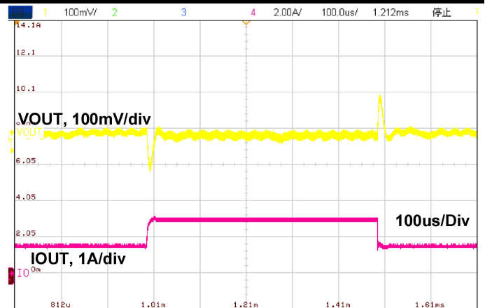
Figure 19. Load Transient, 1.5A-3A-1.5A
