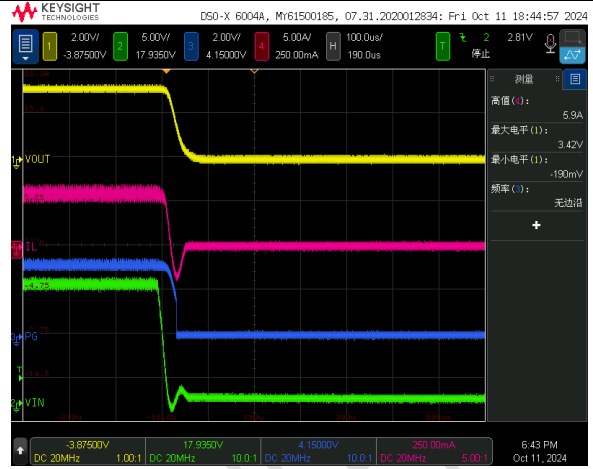
Figure 14. Shutdown by VIN, 6A load
