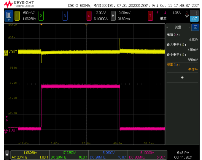
Figure 20. Load Transient, 0.05A-6A-0.05A
