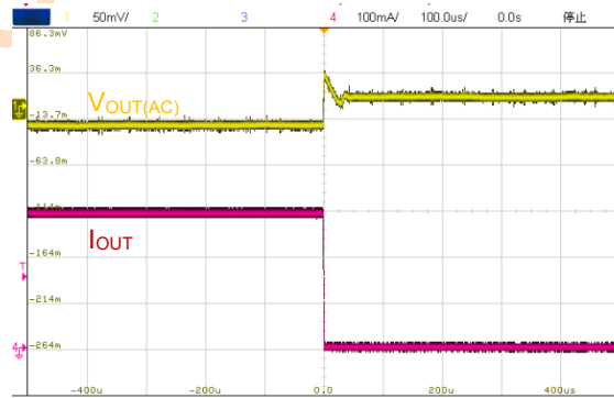
Figure 88 Load transient waveform: I_{OUT}=300\text{mA}\rightarrow 1\text{mA} in 1\mu\text{s}
