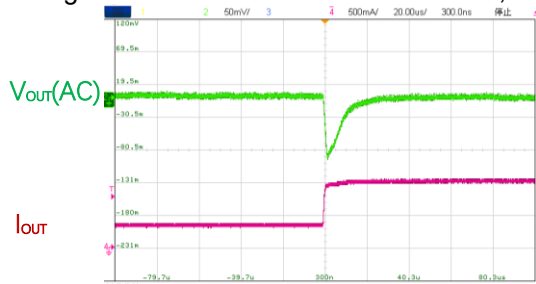
Figure 15. Load Transient 300mA->1A, CFF=0,
