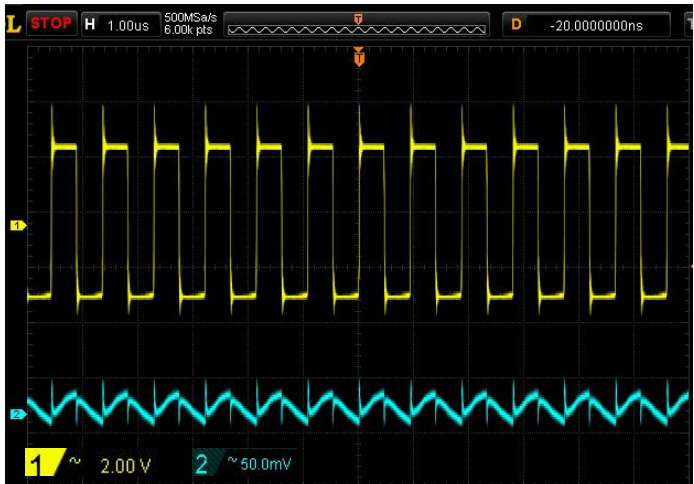
V_{IN}=3V, V_{OUT}=5V, I_{OUT}=500mA, CH_1=V_{SW}, CH_2=\Delta V_{OUT} V_{IN}=3V, V_{OUT}=5V, I_{OUT}=1A, CH_1=V_{SW}, CH_2=\Delta V_{OUT}
