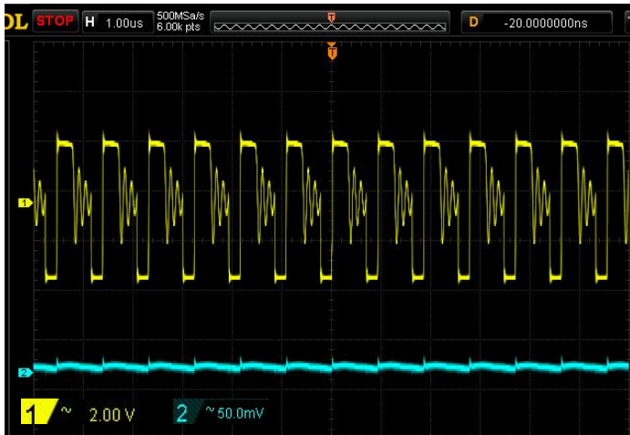
V_{IN}=3V, V_{OUT}=5V, I_{OUT}=50mA, CH_1=V_{SW}, CH_2=\Delta V_{OUT}
