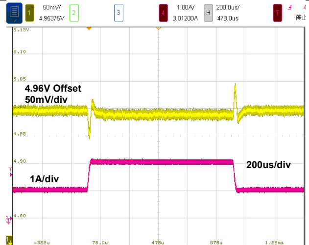
Figure 28. Load Transient, 1A-2A-1A
