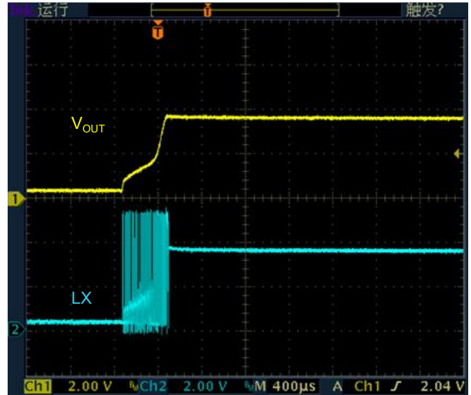
LX waveform @ V_{OUT}=3.3V , Short Output to No Load
