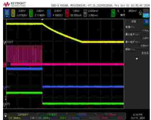
Figure 8. Shutdown by EN, 50Ω load
