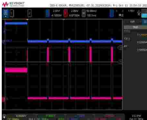
Figure 21. SCP Happen, Hiccup Operation
