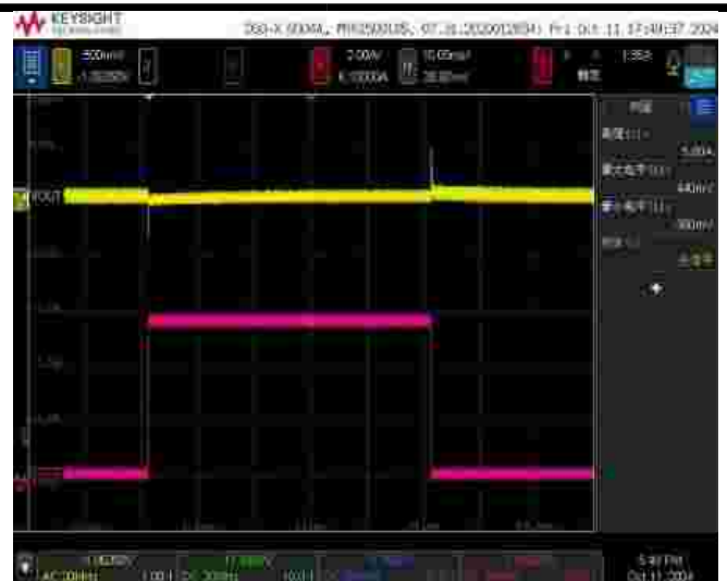
Figure 20. Load Transient, 0.05A-6A-0.05A
