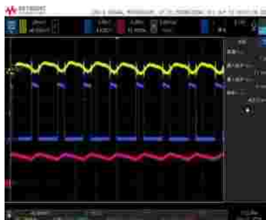
Figure 18. Switching Waveform, 6A load
