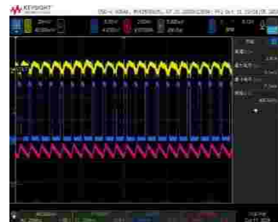
Figure 17. Switching Waveform, 3A load
