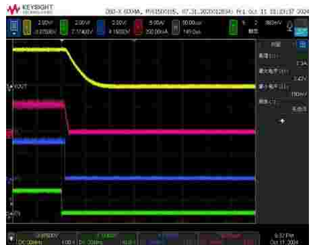
Figure 10. Shutdown by EN, 6A load
