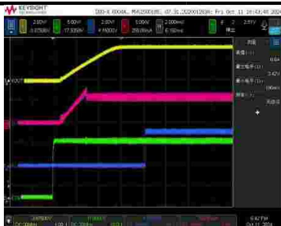
Figure 13. Startup by VIN, 6A load
