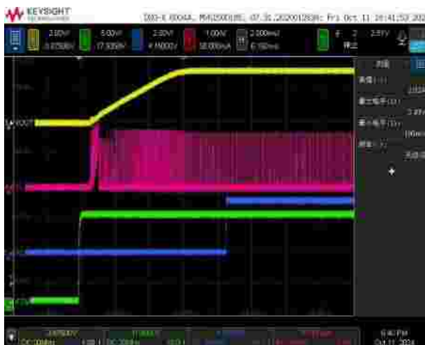
Figure 11. Startup by VIN, 50mA load
